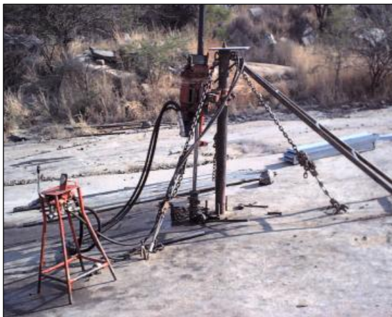
Figure 4 Example of marble stone exploration drill. In this case, drilling takes place on an exposed rocky outcrop, minimising surface disturbances associated with site clearing.
